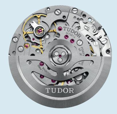
"A high-performance movement, it was crafted in the purest watchmaking tradition, with a column wheel mechanism and vertical clutch."
